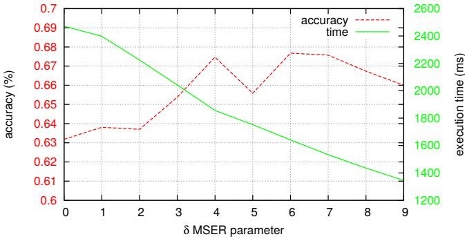
Fig. 7. Analysis of the  $\delta$  parameter of the MSER. The graph shows the resulting accuracy of meter readings and the average execution time for a single input image when varying the  $\delta$  parameter.
