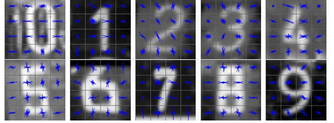
Fig. 4. HOG feature example, one for each class of interest. In this example, each patch  $32 \times 32$  is divided into cells of size  $8 \times 8$  and for each cell the gradient strengths are then visualized by line lengths in the direction of the corresponding gradient bin.
