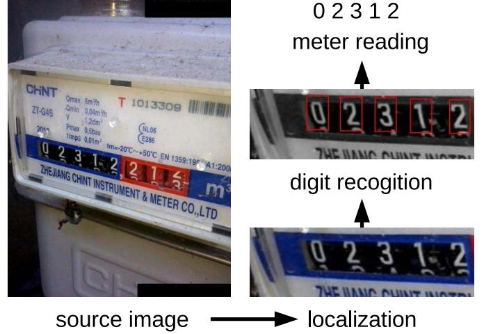
Fig. 1. An overview of the steps performed by the proposed model in order to read the gas meter counter that appear in the source image. The localization phase rotates and cuts the region of interest; the recognition phase identifies all potential digits of interest, while the reading step produces as output the final reading.
