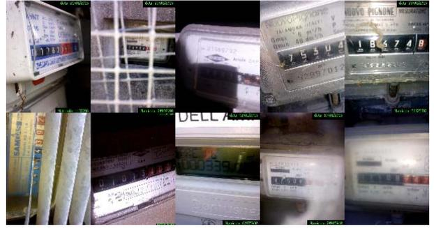
Fig. 9. Some problematic images of the dataset used. In some images the red decimal digits are missing and then the localization fails, while in the others due to poor lighting conditions, occlusions and perspective distortions, the MSER algorithm fails to find the regions containing the digits of interest.
