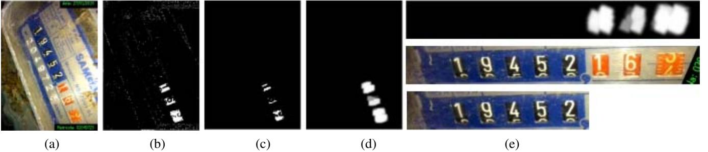
Fig. 3. Gas meter counter localization example. From left to right: source image (a), soft mask of red areas generated by the MLP (b), first (c) and last (d) image of the iterative inflate of the white regions, rotation and crop of the area of interest (e).
