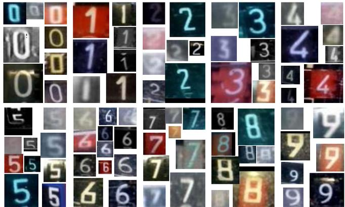
Fig. 6. Training examples of the digit recognition step. From each scaled patch the HOG descriptor is extracted, which become an input pattern to the SVM model. The *not a digit* class is not included and contains regions that do not contain meter's digit.
