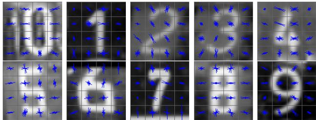
Fig. 4. HOG feature example, one for each class of interest. In this example, each patch  $32 \times 32$  is divided into cells of size  $8 \times 8$  and for each cell the gradient strengths are then visualized by line lengths in the direction of the corresponding gradient bin.
