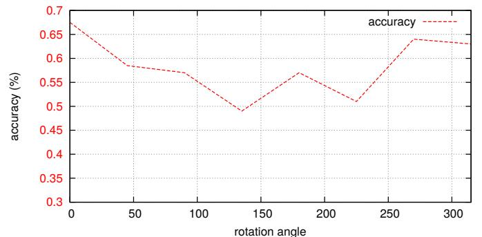
Fig. 10. Analysis of the meter reading accuracy while varying the rotation angle (in degree) of the gas meter counter.
