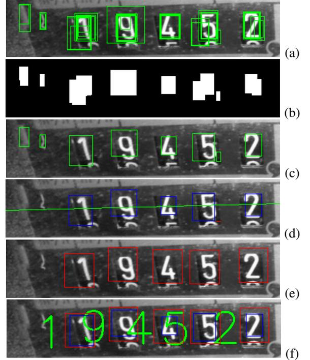
Fig. 5. Meter reading example. From top to bottom: MSER bounding box (a), the activation map (b), the bounding box of the clusters found (c) fit line to eliminate false positives (d), digit hypotheses to eliminate false negatives (e), final reading (f).
