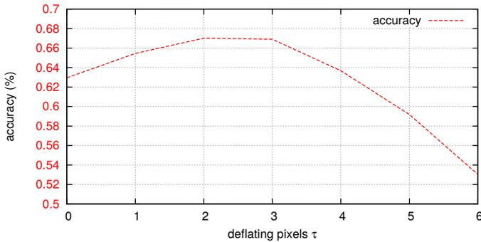
Fig. 8. Analysis of the  $\tau$  parameter, representing the deflating size in pixels of a MSER bounding box  $r_i$ , from which the centroids in the mask  $M$  are identified.
