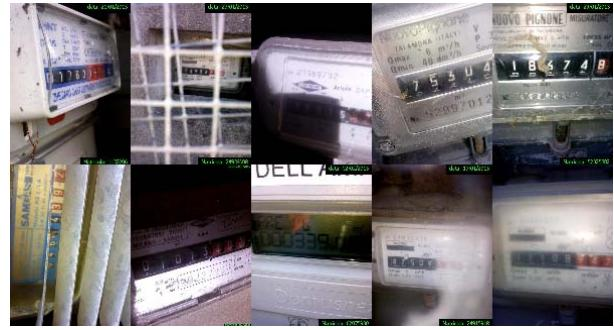
Fig. 9. Some problematic images of the dataset used. In some images the red decimal digits are missing and then the localization fails, while in the others due to poor lighting conditions, occlusions and perspective distortions, the MSER algorithm fails to find the regions containing the digits of interest.
